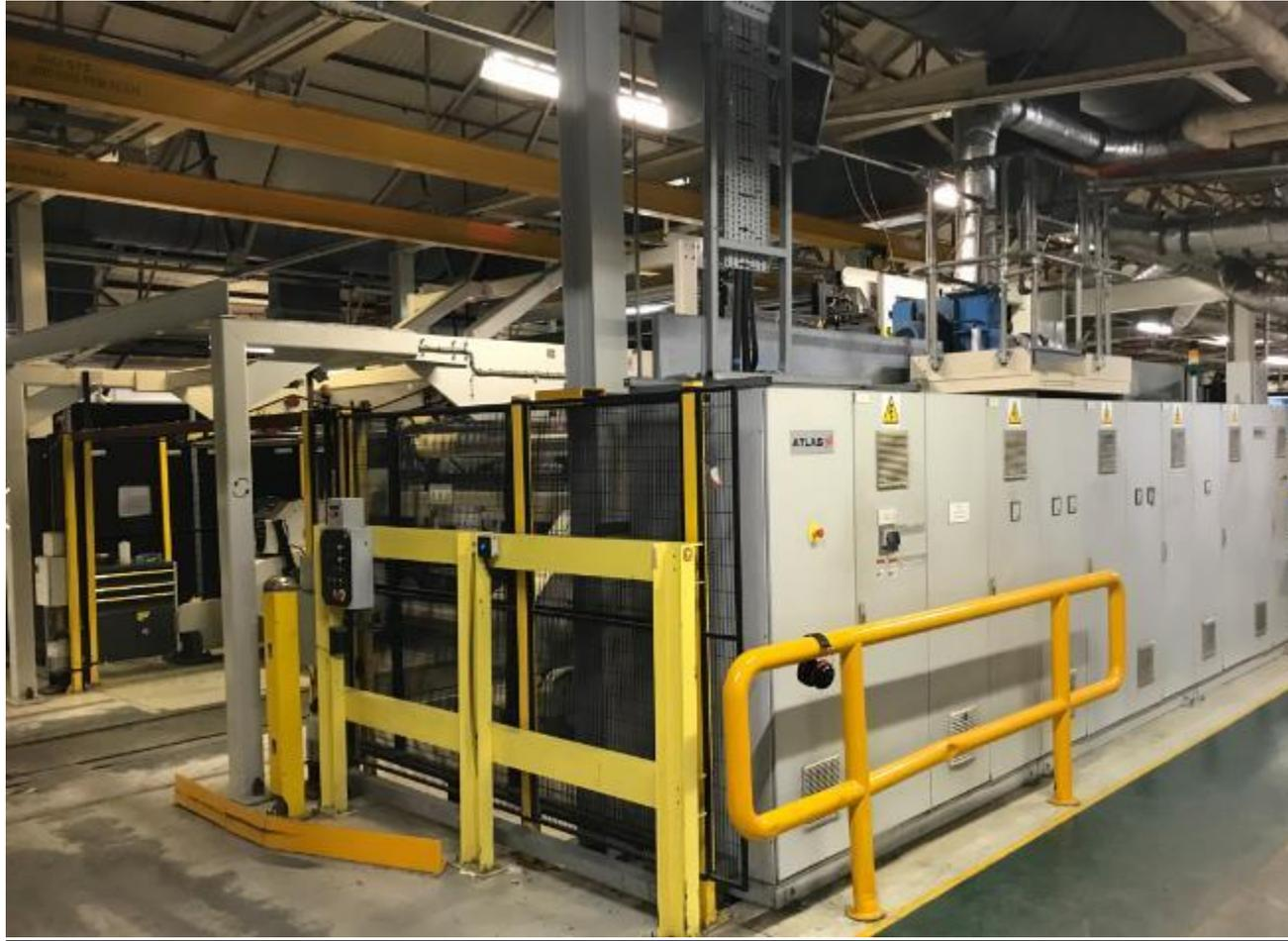
Atlas converting TDW, built in 2006, rated to 415V, 315amps, hydraulic pressure of 155Bar and pneumatic pressure of 6bar. Built to slit banknote paper from 80-200gsm with tension of 8PLI to 1500m/min normal running speed is 1000 Rpm with capability to slit up to seven webs across. Driven unwind which can process max roll diameter of 1500mm with width of 2800mm.
