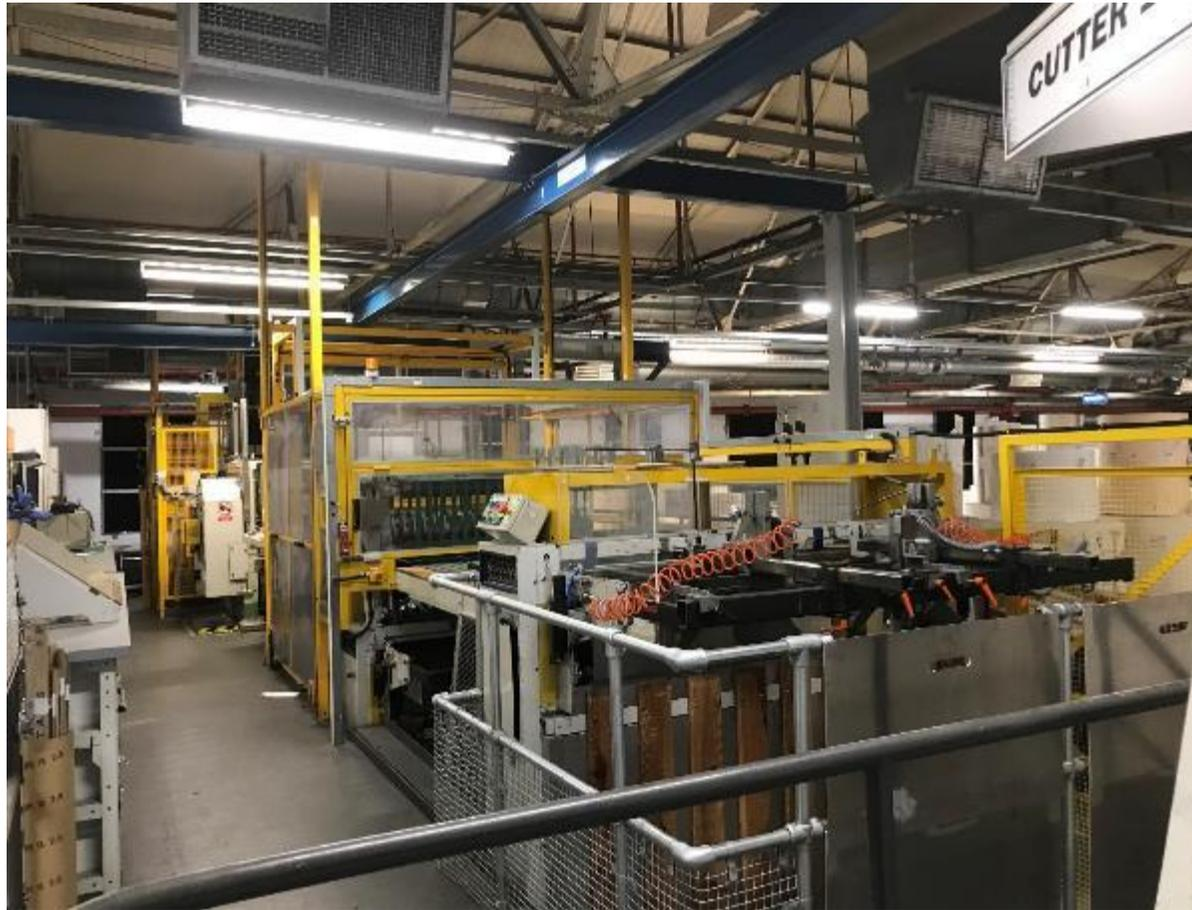
Querschneider Sheeter Type WSKA 1600 Serial no 1551, 415V, 200A, 100Kw, Year 1995 Comes with a Norcan 600-DK series cut to register system, rotary notcher system, ISRA 2017 inspection system, dead knife with PIV gearbox, reject gate and best layboy. Recently upgraded safety control system. Drives on: LH/ Under machine, operator controls: RH, Power cabinets: RH
