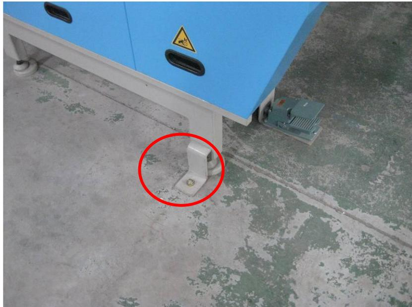
Figure 2-32 Descriptin of Fixing Height Adjustable Feet
