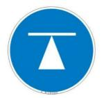
Figure 2-17 Transport point for fork vehicle.
